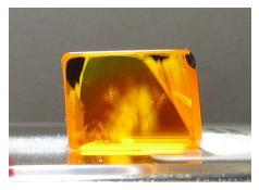
Fig. 6. Bulk damage occurring in the type-I orange phase HGS-1 OPO element generating 4  $\mu$ m idler pulses after using it for hours at ~95 mJ pump energy and 100 Hz.
