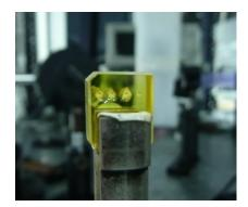
Fig. 11. Rear surface crack observed in CGS.
