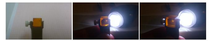
Fig. 8. Surface damage on the HGS-2 OPO element generating 6.3 µm idler pulses at 140 mJ pump energy and 10 Hz.
