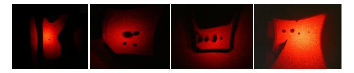
Fig. 10. Crystal shadow patterns for HGS-Y, HGS-O, CGS, and CHGS (from left to right) each with 4 damage spots.
