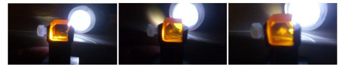
Fig. 7. Bulk damage occurring in the type-II orange phase HGS-2 OPO element generating 6.3  $\mu$ m idler pulses after using it for hours at >100 mJ pump energy and 10 Hz.
